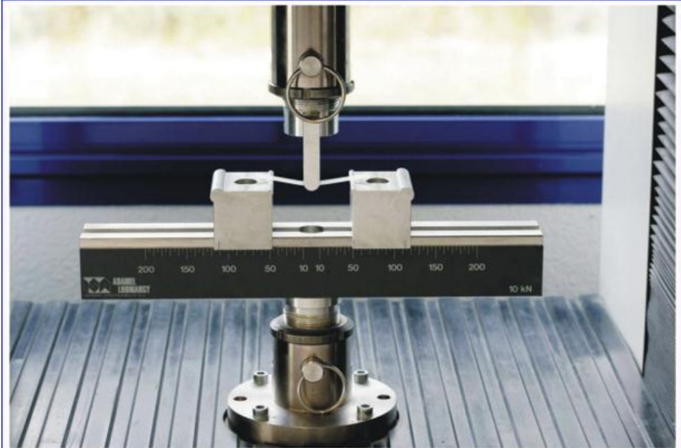
Image 4 of 8 Figure 2. Flexural strength test conducted according to ISO standards.
